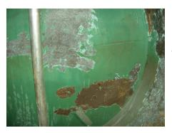
The lining (green) is peeling off the inside of this UST and the tank walls are rusting.
